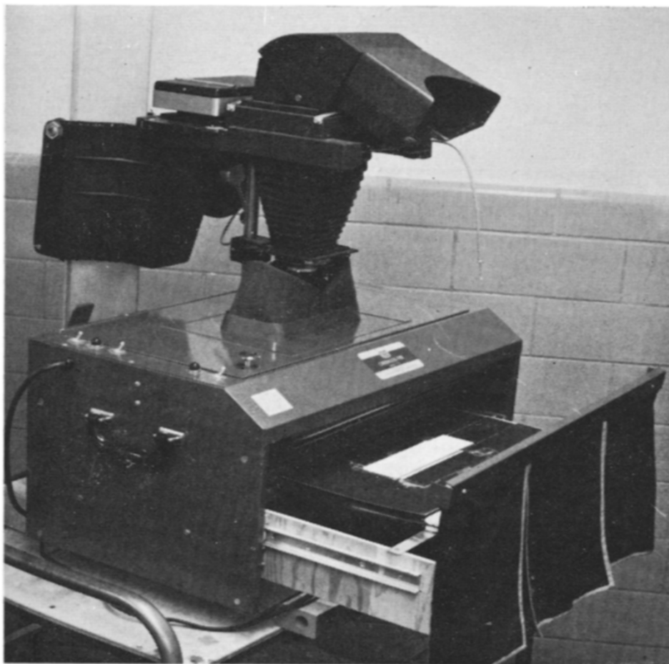
Fig. 1. Fluorescence Analysis Cabinet modified to permit photography with the MP-3 camera as well as inspection of chromatograms under ultraviolet radiation and to permit inspection by means of transmitted and reflected white light.
